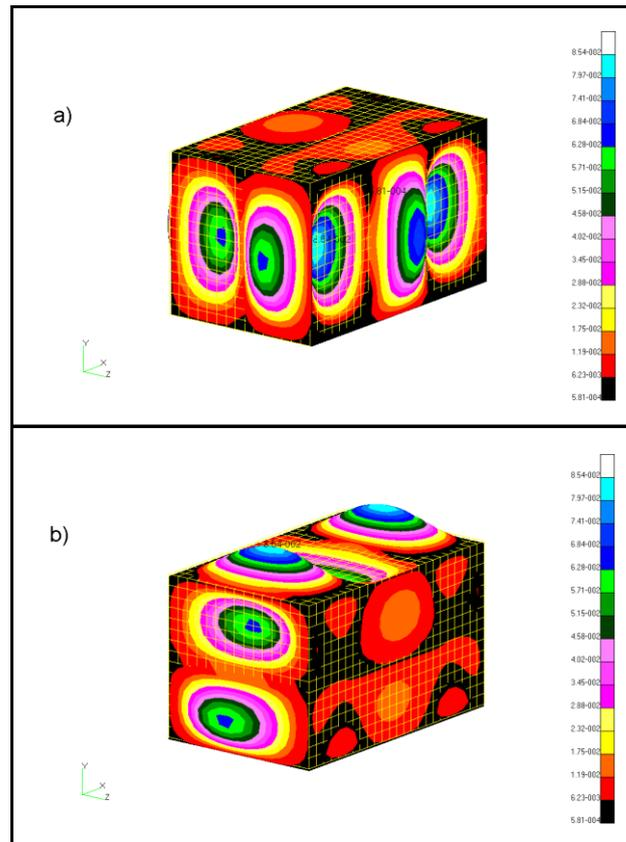
Fig. 5. ‘Waveguide modes’ of a modified box model ‘A’ at 42.36 Hz in the directions of:
