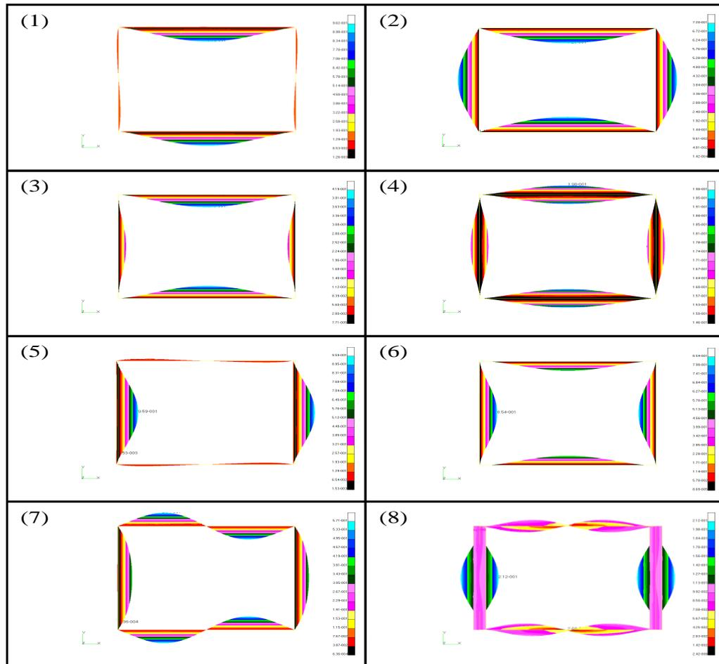
Fig. 8. First eight normal modes calculated for Dickinson and Warburton's model in XY plane
