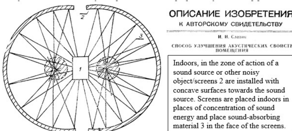
Fig. 2. The Slavin patented device for sound absorption (Edited from [6])
