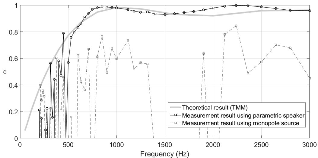
Fig. 3. Measurement and simulation results for the glass wool
