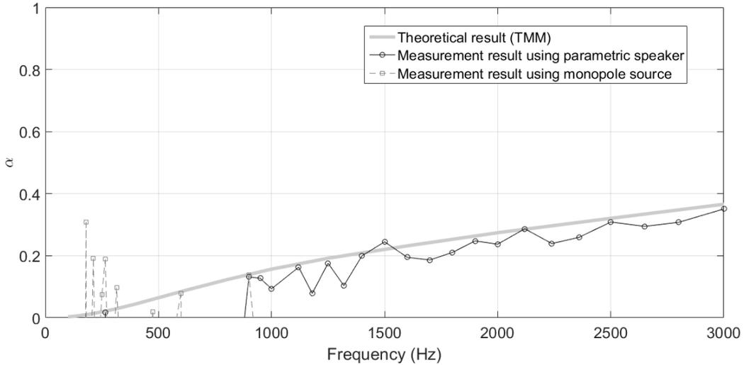
Fig. 6. Measurement and simulation results for the 0.5 in. thick melamine foam
