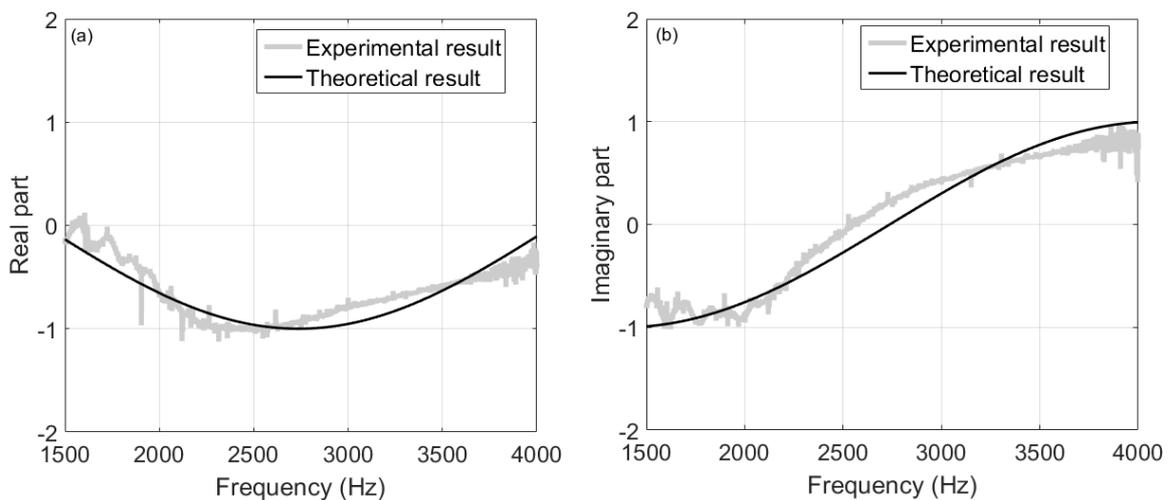
Fig. 8. Measurement and simulation results for the honeycomb panel – Reflection coefficient for a 10° incidence angle
