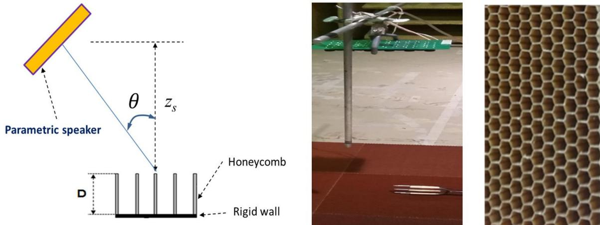
Fig. 7. (left) Sketch of the measurement setup – (middle) picture of the parametric speaker and measurement microphones installed above the honeycomb structure – (right) close-up view of the honeycomb
