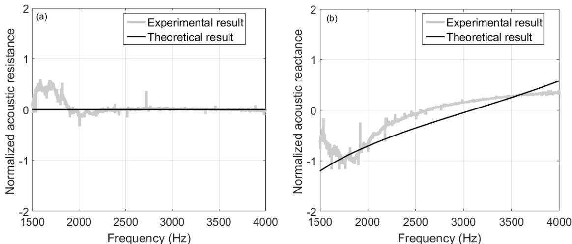
Fig. 9. Measurement and simulation results for the honeycomb panel – Normalized surface impedance for a  $30^\circ$  incidence angle
