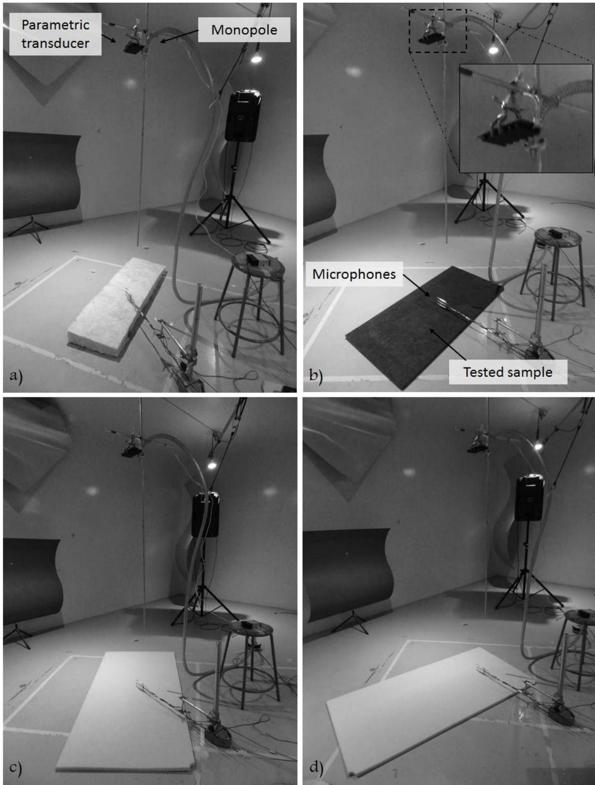
*Fig. 2.* Pictures of measurements in the reverberant room – a) Glass wool – b) Compressed glass wool panel – c) Melamine foam, 1-inch thick (position 1) – d) Melamine foam, 1-inch thick (position 2)
