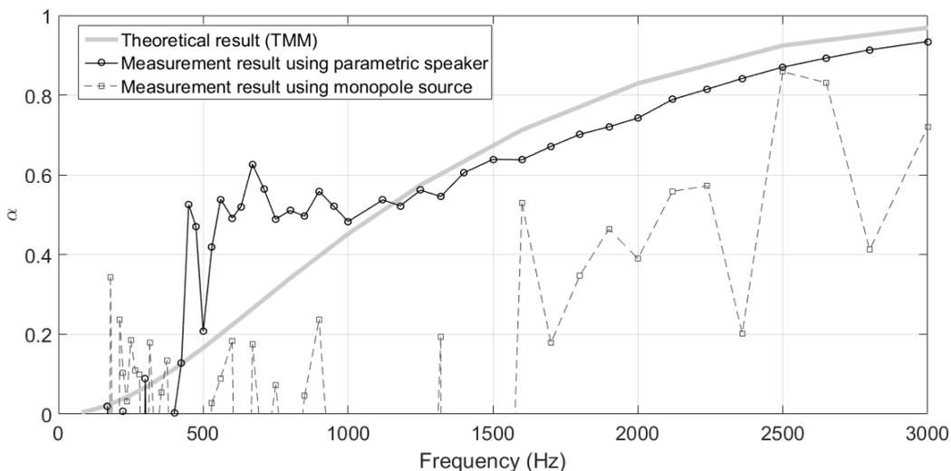
Fig. 4. Measurement and simulation results for the compressed glass wool panel
