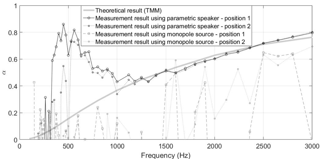
Fig. 5. Measurement and simulation results for the 1 in. thick melamine foam
