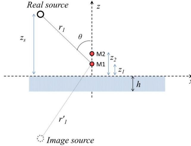
Fig. 1. Typical two-microphone experimental setup based on an image-source model
