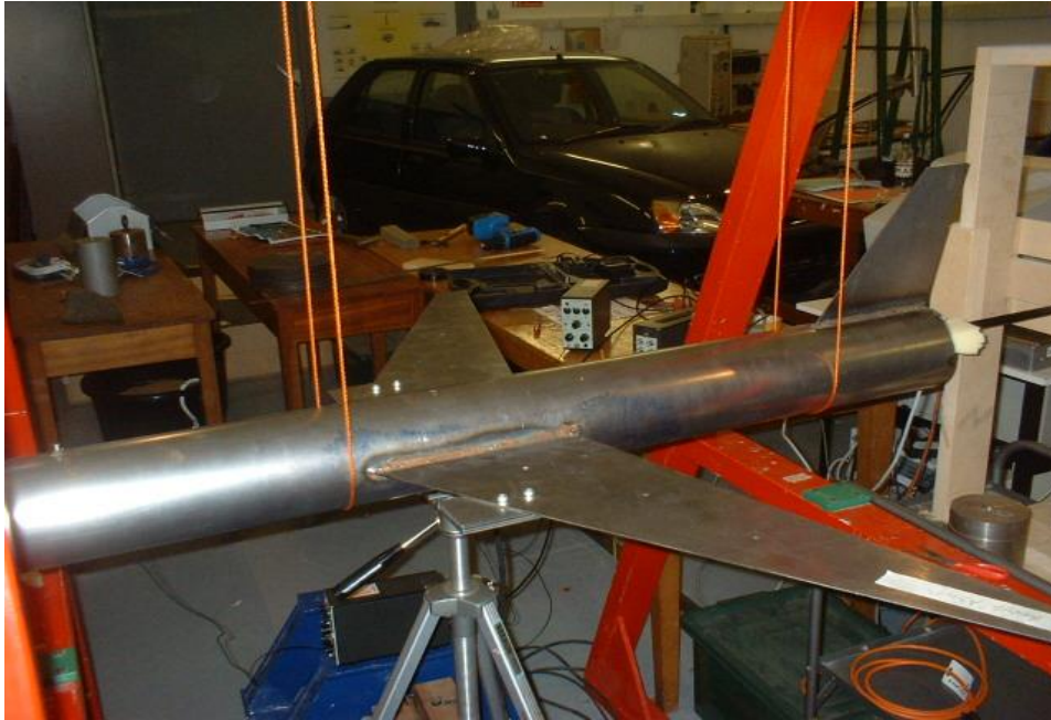
Fig. 3. The manufactured reduced-scale aircraft model supported by suspensions
