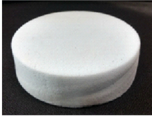
Fig. 3. Impedance tube foam test sample of 100 mm diameter with 22 mm thick
