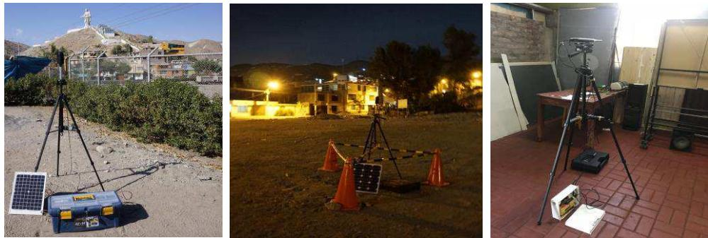
Fig. 1. Pictures of medium and long term outdoor and indoor monitoring stations
