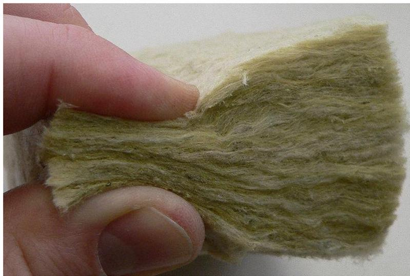
*Fig. 1.* Porous materials obtained from mineral wool [13].
