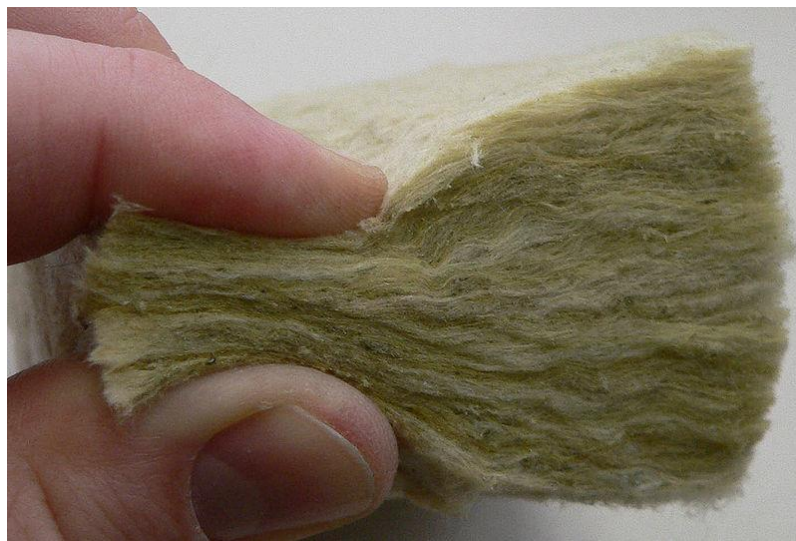
Fig. 1. Porous materials obtained from mineral wool [13].
